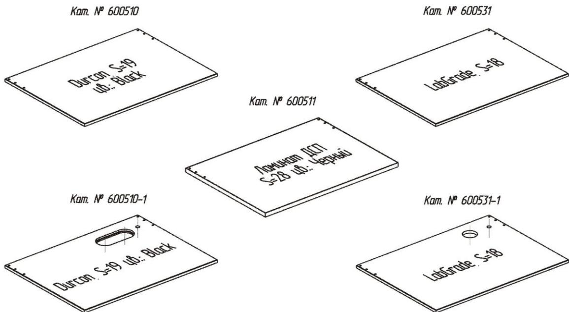
Table tops made of laminated chipboard have durable plastic edge of 2mm thick.
