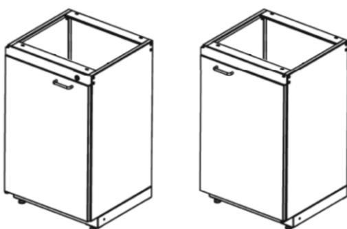
Washer pedestals differ from conventional ones in reinforced frame and the lack of locks.
