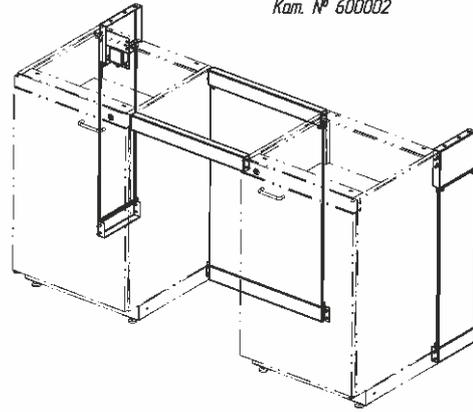
Complete sets are necessary for connecting pedestals and frame tension clamps. Complete set also includes decorative screens to close the technological sections and fittings for tables assembly.
