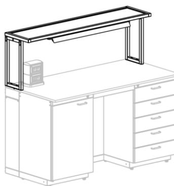
All racks in the Inova series are equipped with fluorescent lights with screens.
