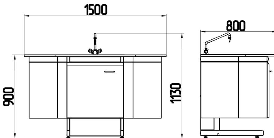
The service compartment takes the entire volume under the washer, thereby providing excellent access to services. Storage compartments are located on the right and left of the door, in aprons.
