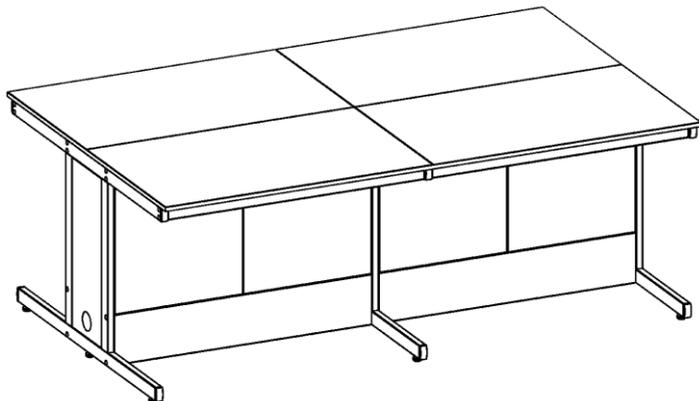
Island table tops consist of 2,4 or 6 pieces (depending on the amount of sections), which allows to replace only the damaged piece in case of destruction of the working surface.
