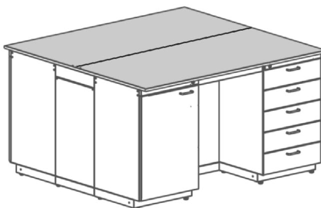
Table tops of island tables are joined together out of two side table tops. Table tops can be combined at will, but be careful: when joining LabGrade and Durcon table tops with laminate ones, the ledge of 10mm thick between different table tops is unavoidable.
