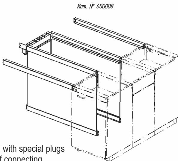
Decorative panels of island tables are equipped with special plugs of large diameter which can be removed in case of connecting services to island tables.
