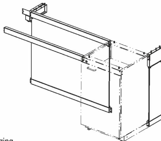
Additional side sections are designed for maximizing space for legs at seated activity.
