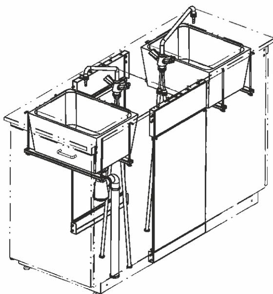
Components of tables with sinks, in addition to screens, fasteners and ties include drain sinks with sanitary equipment and mixer taps with flexible connections.
